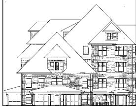
Partial elevation of proposed apartments at East Broad and Twenty-Second Street follows many of the design guidelines. The massing of this lengthy building is broken by varied rooflines and stepped setbacks.
