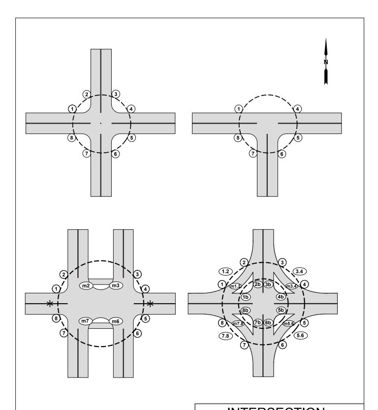
ALL NUMBERING BEGINS FROM THE NORTHWEST CORNER AND GOES CLOCKWISE. EACH CORNER HAS ITS SPECIFIC NUMBER THAT SHALL BE USED IF CURB RAMPS ARE IN THESE LOCATIONS.
