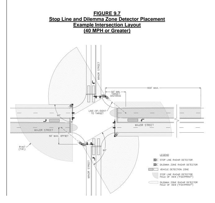
The preferred mounting location for dilemma zone detector units shall be on the signal support on the near right corner of the subject approach to the intersection as shown in **Figures 9.7** and **9.8**.
