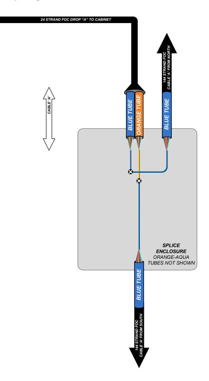
Figure 12.14 Splicing Orientation – 3 Cables
