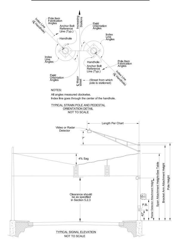
Figure 4.4 Typical Strain Pole Fabrication and Orientation Data
