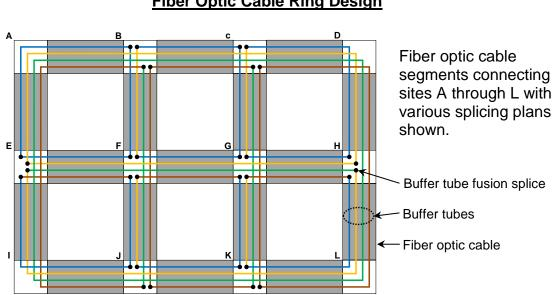
Figure 12.6 Fiber Optic Cable Ring Design
