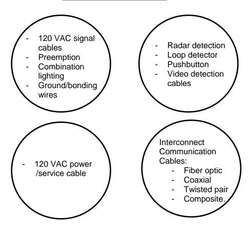
Only cables serving traffic signal elements mounted on a signal support shall enter the base/foundation of that structure. All other cables shall bypass the foundation. Traffic signal cable should not loop through a signal support structure when that cable does not serve devices on that support.
