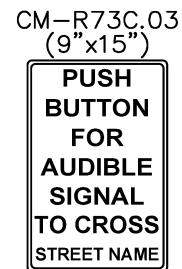
Figure 6.4 Audible Pushbutton Sign
