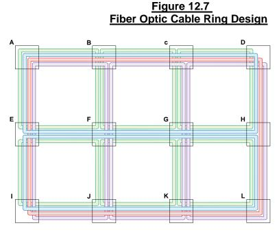
Physical optical pathway of fiber tubes, as spliced in Figure 12.6, create green, blue, red, and purple 'rings'. This color scheme is completely arbitrary and may be composed of various fiber/buffer tube color combinations.
