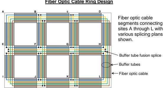
Figure 12.6 Fiber Optic Cable Ring Design
