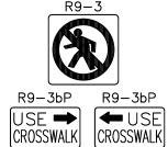
"Use Crosswalk" R9-3bP (18 in. x 12 in.) plaque shall be placed under the No Ped Crossing sign and shall have an arrow directing pedestrians to the nearest crossing.
