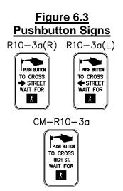
pushbuttons located at the side of the landing area, sign R10-3a shall be used. If the pushbutton is located at the back of the landing area, sign CM-R10-3a shall be used.
