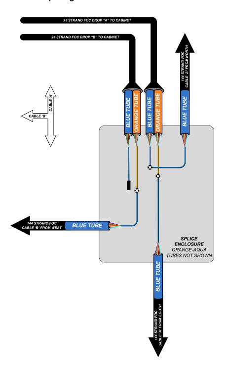
Figure 12.15 Splicing Orientation – 4 Cables
