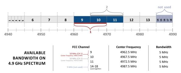
Figure 12.16 4.9GHz Frequencies Available for Signal Interconnect Communication
