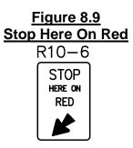
The sign post should be centered on the stop line and placed as close as possible to 3 ft. behind the curb or 6 ft. off of the edge of pavement.
