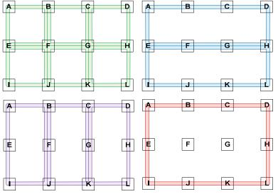
Individual fiber tube rings are broken out showing which sites have access to each respective tube.
