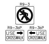
"Use Crosswalk" R9-3bP (18 in. x 12 in.) plaque shall be placed under the No Ped Crossing sign and shall have an arrow directing pedestrians to the nearest crossing.
