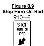
The sign post should be centered on the stop line and placed as close as possible to 3 ft. behind the curb or 6 ft. off of the edge of pavement.
