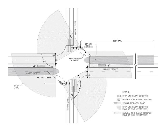
The preferred mounting location for dilemma zone detector units shall be on the signal support on the near right corner of the subject approach to the intersection as shown in **Figures 9.7** and **9.8**.
