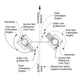
All angles measured clockwise. Base plate is oriented square to Mast Arm.
