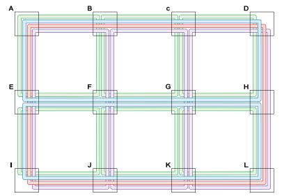
Physical optical pathway of fiber tubes, as spliced in Figure 12.4, create green, blue, red, and purple 'rings'. This color scheme is completely arbitrary and may be composed of various fiber/buffer tube color combinations.
