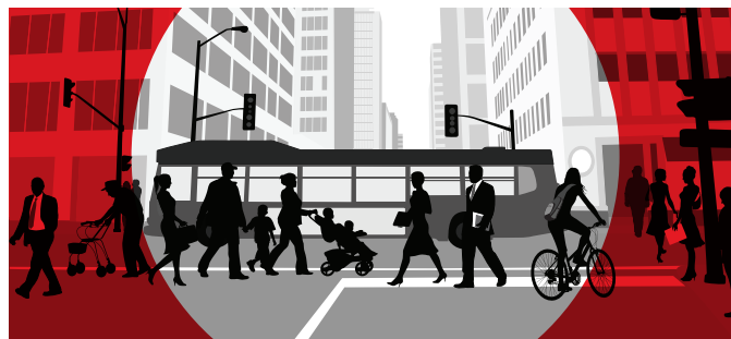
Driver field of vision at 30 MPH. A pedestrian's risk of death is 40% if hit at this speed.
