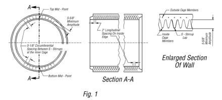
Illustrative Example of S-Stirrup Support System for 0.01-inch Crack D-load 3000, 102-inch diameter Pipe Minimum Area Per Support 0.053 square inch, 11 Lines Spaced @ 5 1/8 inches. For other classes and sizes, see Tables 706.02-2, 3, and 4.
