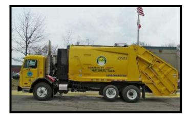
The division put its first Hydraulic Launch Assist (HLA) assist truck into service. HLA technology is designed to improve both fuel efficiency and overall operating economy of vehicles.
