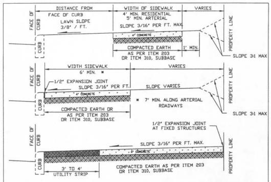
SIDEWALKS SHALL BE CONSTRUCTED WITH P.C. CONCRETE (CLASS C, ITEM 499) WHICH SHALL CONTAIN 5% TO 8% ENTRAINTED AIR AND A 3" MAXIMUM SLUMP.
