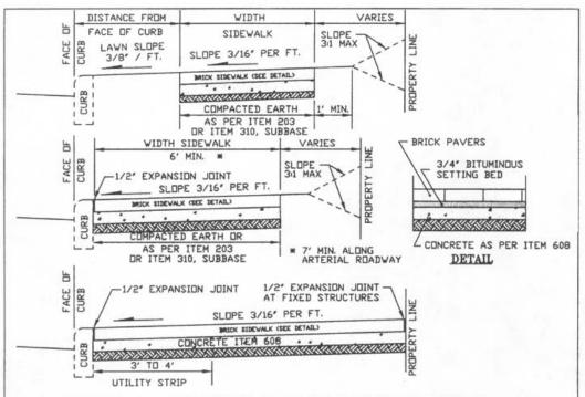
SIDEWALKS CONSTRUCTED WITH P.C. CONCRETE(CL.G,ITEM 499) WHICH SHALL CONTAIN 5% TO 8% ENTRAINED AIR AND A 3" MAXIMUM SLUMP.
