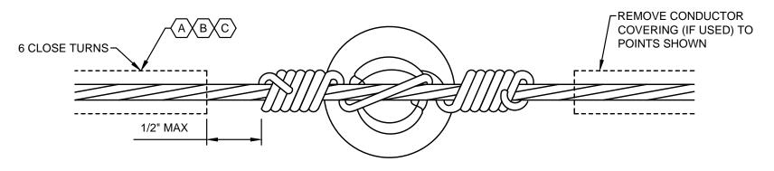
DETAIL 1 **TOP GROOVE TIE - SHORT SPAN**
