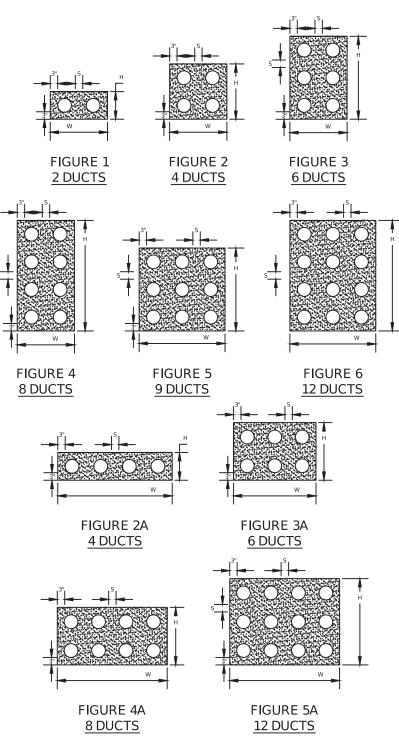
Figure 3004-1: Typical Duct Bank Configurations
