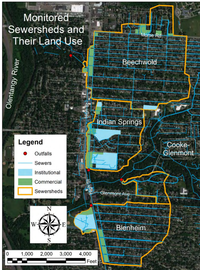
Figure 2. Boundaries of the four monitored sewersheds (orange) and land use within each sewershed. Commercial and institutional land uses are shown in blue and green polygons, respectively. All remaining land within each sewershed was residential.
