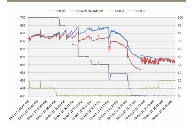
Note the large manual corrections to DSR 83 level through regulator gate movements.
