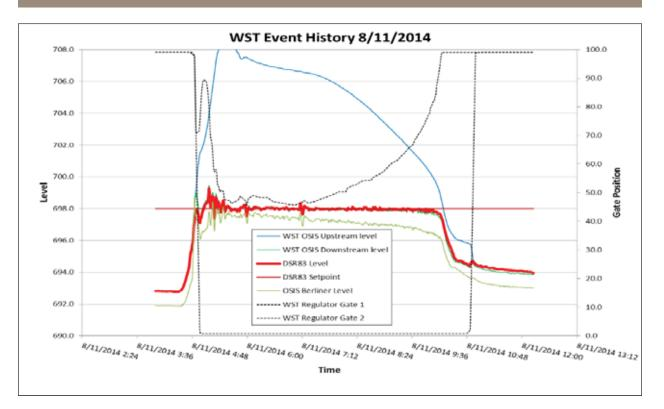
Note the small continual automatic corrections to DSR 83 level through regulator gate movements to maintain the DSR 83 698-foot set point.
