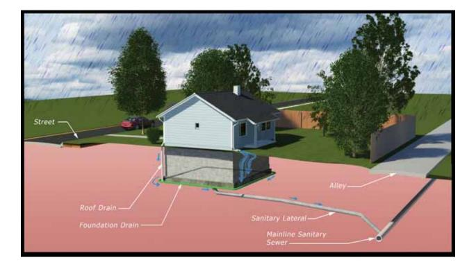
The inflow source shown in Exhibit 6.1.2 is a roof drain (downspout) that is directly connected to the foundation drain. This connection rapidly fills the foundation drain with rainwater and enters the private sanitary lateral feeding the sanitary sewer. This connection was made illegal in 1907. The city's I/I studies have found that these connections are relatively rare.
