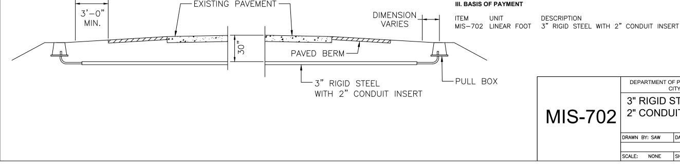
A. THE 3" RIGID STEEL CONDUIT SHALL BE HOT DIPPED GALVANIZED AND SECONDARY COATED PRODUCED TO ANSI SPECIFICATIONS C-80.1 AND MEET REQUIREMENTS OF UNDERWRITERS LABORATORIES UL-6. BOTH ENDS SHALL BE THREADED. THE CONDUIT SHALL BE OMEGA TUBE
